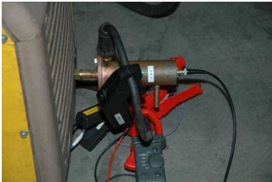
Figuur 11: meetopstelling (shunt + stroomklemmen)
